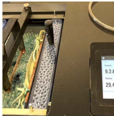
Through-hole plating process
