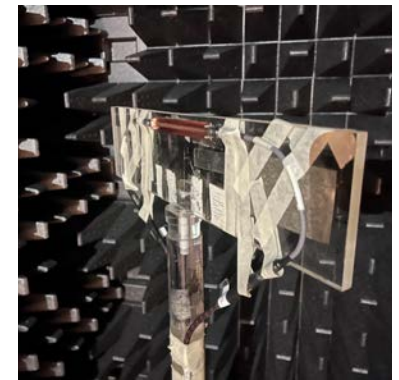
S-parameters and far-field measurements in anechoic chamber
